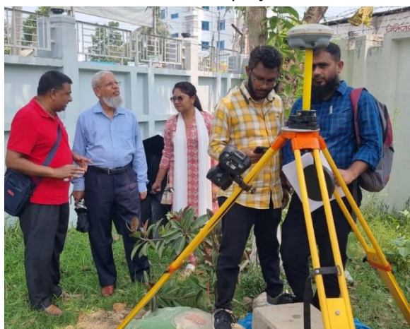
RTK Base setup going on
